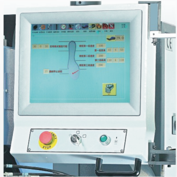
伺服送膠系統精確掌控多段膠量 servo-motor feeding system controls precise cement quantity for each sections.
