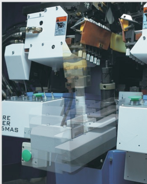
電腦自動控制並記憶撐台上下位置 Computerized automatic programmable and memorized height position of last supporter
